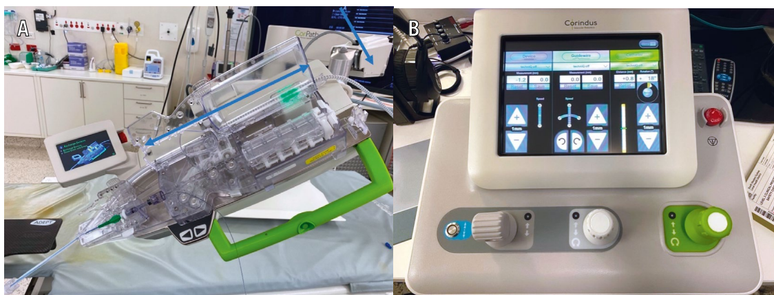
Figure 1. Robotic setup. Reproduced with permission from Dr J Leung.. A) Bedside console with robotic drive. B) Shielded operator cockpit with touchscreen and three joysticks to control the catheter, guidewire, and cardiac device.
