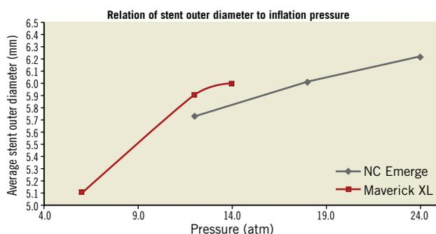
**Figure 3.** The relation of the change in stent diameters to pressure used for stent expansion using 6.00 mm balloons (SC Maverick and NC Emerge). Very high pressures were required to overexpand the stents at 5.5 to 6.0 mm diameters. The preserved radial strength of the SYNERGY allows it to be post-dilated with a 6 mm balloon to RBP without fractures. Note: Maverick XL RBP=14 atm; NC Emerge RBP=18 atm.
